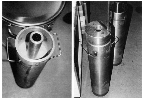
Fig. 1. Photograph of a large-scale hollow capsule. Outer diameter: 147 mm and inner diameter: 32 mm.
